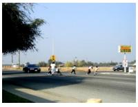
Reducing the number of traffic lanes will allow installation of a median for pedestrian refuge.
