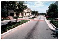
The bulb out and median in the photo above depict the type of design Phase One: recommended on Avenue 416. The median provides a refuge for people crossing, whether at the school or near shopping. Crossing distance is greatly reduced by the median, the reduction in lanes, and the bulb out. Stop lines in advance of the crosswalk should also be used.
